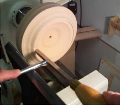
Figure 1 – Secondary Tool Rest in Use with a Bedan.
