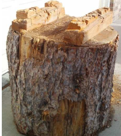
Figure 3 – Stump Saw Horse
