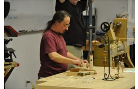
Mike demonstrates the beginning steps of marking the stock and drilling the holes.
