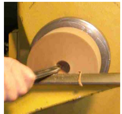
Notice how he moves from the center to the outside rim, to follow the grain.
