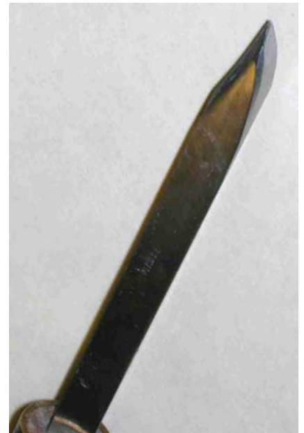
Samples of Bruce's tools, with close-ups of the bevels and curves. He's given them a reverse chamfer for use in scraping in tight corners.
