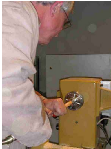
Boring out stem for lamination. Be sure to back out to clear shavings.
