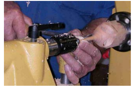
Steve predrills the holes using Forstner drills on a drill press. Once mounted, he turns the basic shape of the top, and then turns the finial.
