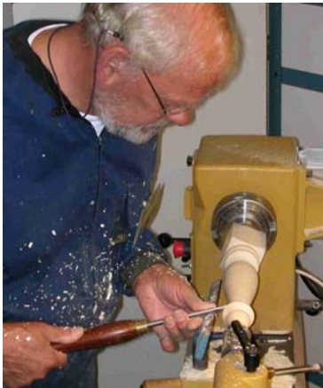
Chris showing how to turn a table leg. The challenge is making them all match!
