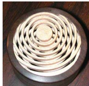
Example showing the eccentric side up. Also note the piece is inlaid into a solid wood rim to help hide where the cuts exit the sides of the piece.
