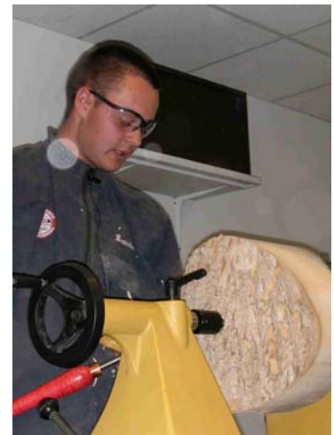
Brandon starting to round his log cutout. The log is mounted on a faceplate and the tailstock is being used to steady the wood. He roughs out with 3/8" bowl gouge.
