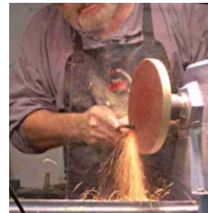
MDF disk with metal-cutting sandpaper disk used to grind shape of O1 drill rod steel.
