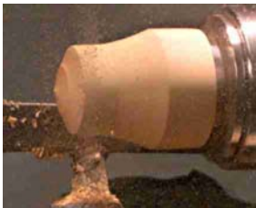
Box in process, turned completely with skew.
