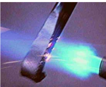
Reheating bent tip to get ready for tempering. After tip glows cherry red, douse in olive oil in metal can. Stir tip to disperse heat. Be careful of potential fire hazard – have an appropriate fire extinguisher or metal lid to smother fire. After
