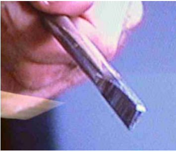
Close-up showing ground shape with wedge. The narrow edge will be the cutting edge.
