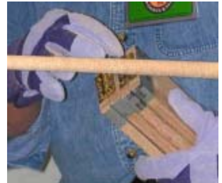
John's sanding tools – sandwich blocks with different grades sandpaper and loose hinges to allow blocks to ride taper.
