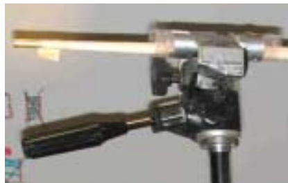
Closeup of John's "tailstock" – pipe mounted to a camera tripod and the rod allowed to spin freely.
