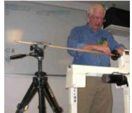
Showing John's full setup. Butt end of rod is clamped in chuck jaws. Tapered end is fed through pipe on tripod. John never turns on lathe without steadying the rod to ensure that it doesn't start whipping.
