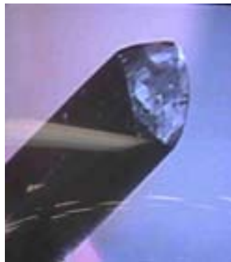
Close-up of the "multi-faceted" grind he uses on his gouges.
