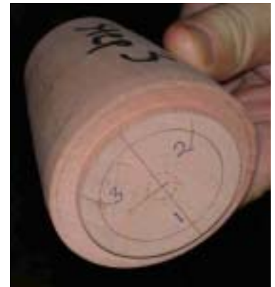
Blank showing chuck tenon turned to first diameter
