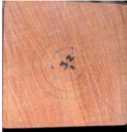
Transferring the marks to the blank. Narrow end of taper.
