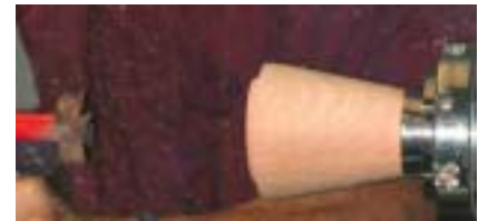
Blank mounted to turn taper and chuck tenon.
