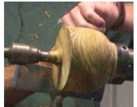
Starting spike, with tailstock as support.
