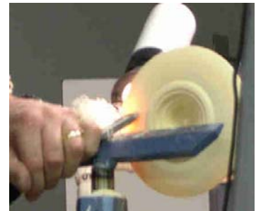
Backlighting to help guide thickness.
