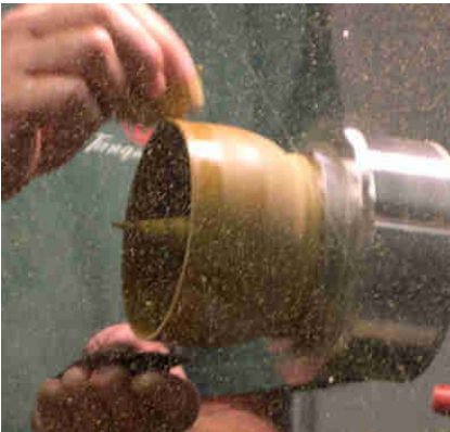
Finishing inside before remounting to turn bottom.
