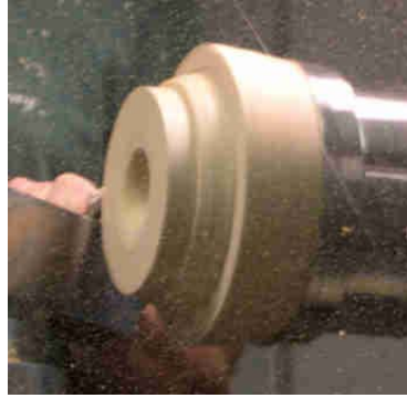
Turning jam chuck to remount. Be sure to leave room for spike!
