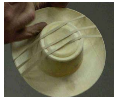
Backlighting to help guide thickness.
