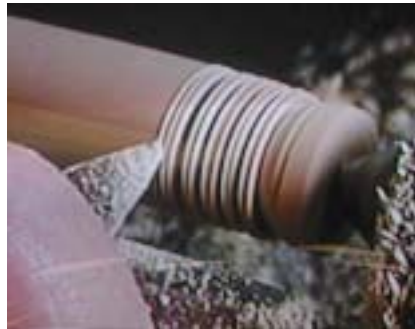
Parting rings for captured rings.
