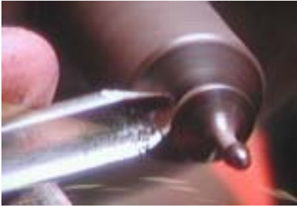
Using gouge to turn lid of small lidded box.
