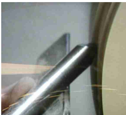
Close-up of how his gouge rides during the push cut. Stuart grinds all his bevels to 40 degrees – the angle of a beaver's tooth (why argue with nature's best woodworker?).
