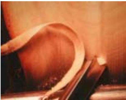
A close-up view of where on the gouge the wood is being cut while turning the exterior of the bowl.
