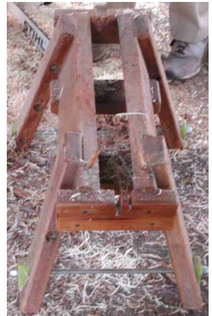
Picture of Gene's bucking stand. It is shaped like a slanted sawhorse with the top supports separated. Note the two wooden dowels in the front to keep the log in place.
