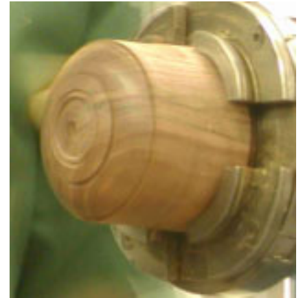
Close-up of the outside of the form. Note the turned tenon so the blank can be reversed in the chuck and hollowed.
