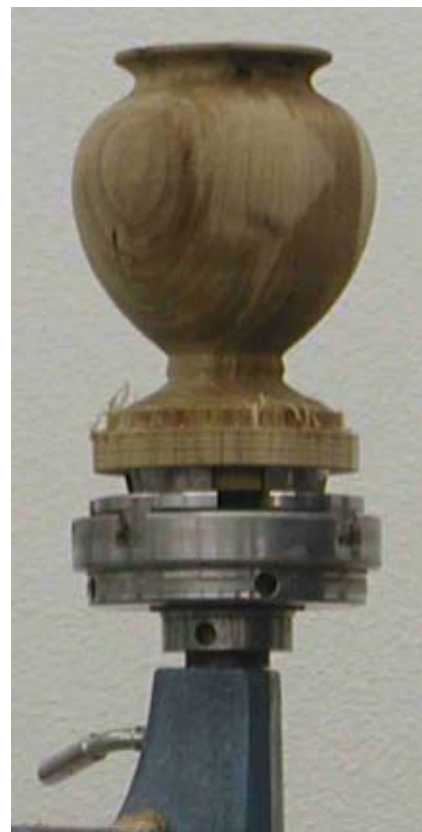
Trent likes to carve his bowls while still mounted in the chuck.
