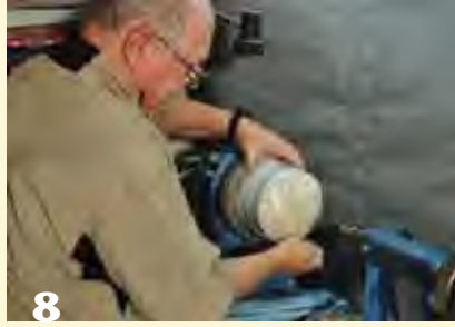
8 Mount the completed compliant vacuum mandrel assembly onto the lathe spindle. You might need Teflon tape on the spindle threads for a good vacuum seal.
