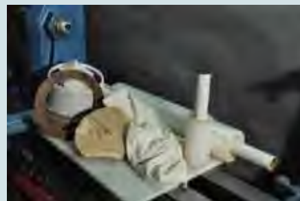
Loosely confining the rice in cloth bags makes it easier to handle and less of a mess in the event of membrane failure.
