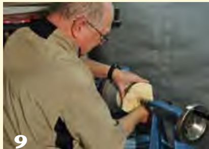
9 Press the burl blank into the plastic film and the rice. The compliant surface molds itself to fit the surface of the burl. Bring up the tailstock to help position the blank and hold it in place.
