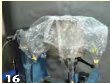
16 Remove the rubber band and spread the film down and around the vacuum chuck.
