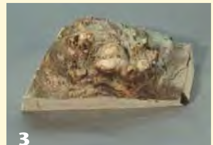
3 To demonstrate the technique, this burl blank is to be turned without damaging the gnarled bottom surface. Like coffee in a vacuum-packed bag, the rice is hardened by the vacuum to the shape of the turning.
