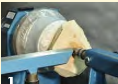
1 The compliant vacuum mandrel, with pressure from the tailstock, cradles the burl for rough turning and shaping the outer rim. The mandrel consists of plastic stretch film over a conventional vacuum chuck that is filled with rice.
