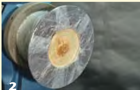
2 The compliant vacuum chuck uses a force ring to hold the blank around its rim, providing unobstructed access for hollowing. The ring wrapped in shrink film presses the turning into the rice-filled vacuum chuck.
