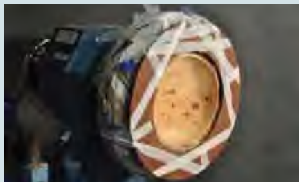
A protective ring taped onto this compliant vacuum chuck protects the plastic film from accidental cuts by the turning tools.
