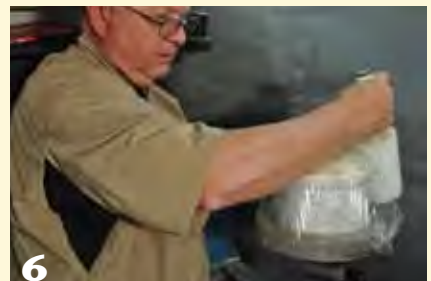
6 Wrap plastic stretch film around and over the surface of the rice and the chuck. Wrap the film in a crisscross pattern so it overlaps and covers all surfaces. The film stretches and clings to itself and the chuck, forming a vacuum-tight seal.
