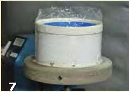
7 Wrap a couple of layers of film that extend up beyond the rim to help nestle extra rice around the burl later in the process.
