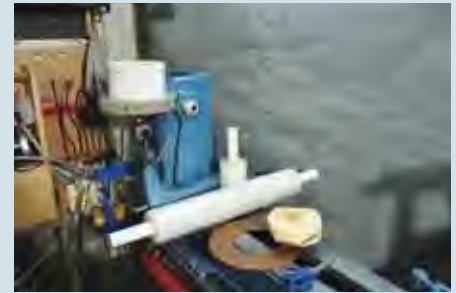
The compliant vacuum chuck requires two widths of stretch film, plus a plywood force ring. The standard vacuum chuck mounted on the carving stand is filled with rice. The burl turning at right is partly complete thanks to the compliant vacuum mandrel.
