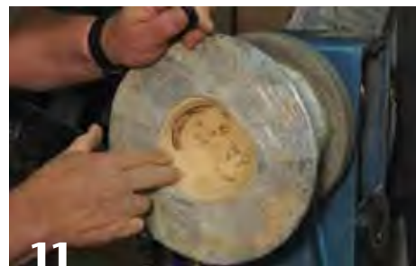
The compliant vacuum chuck retains the turning with a plywood force ring wrapped in plastic stretch film. The vacuum pulls the force ring and the turning into the rice-filled mandrel.
