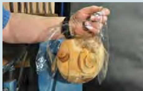
When a blank leaks air, try placing plastic food wrap over it. Before applying the film to this green-turned crab apple bowl, the vacuum level was 4" Hg; with the film smoothed out and taped down at the edges, it increased to 19" Hg.
