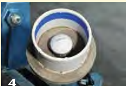
4 The vacuum chuck is ready for filling with rice. The white dome in the center is a 2" (5 cm) PVC pipe cap fitted into a groove cut into the base of the chuck. It has four ½" holes drilled around the perimeter to allow airflow into the spindle. A shopmade filter keeps the rice out of the spindle.
