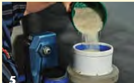
5 Grains of rice poured into the chuck will support the plastic film and the burl blank. The vacuum will draw the loose grains into a solid mass.
