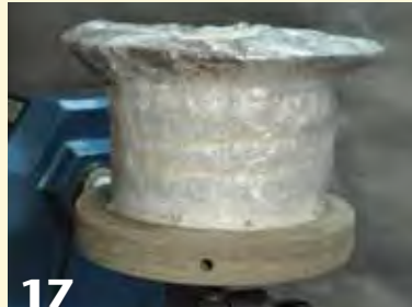
17 Smooth the plastic stretch film around the sides of the vacuum chuck, and hold it in place with a rubber band. Trim the film to the rubber band.
