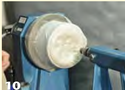
10 Removing the burl while leaving the vacuum switched on reveals how the film and rice conformed to its gnarly surface.
