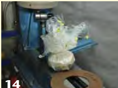
14 Gather the large square of film around the turning blank and hold it with a rubber band.
