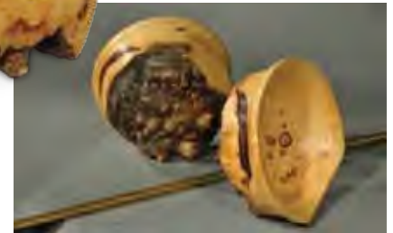
A new technique, compliant vacuum chucking, enables turning gnarly burls like this without having to cut into the rough surface.
